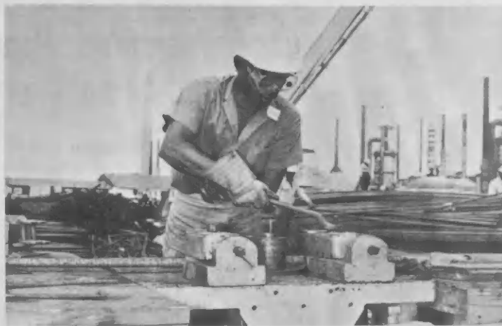
At the RE-BAR bending machine a Parsons employee wears goggles, heavy canvas gloves and apron for protection.
